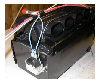
Route wire harness across top of the evaporator and attach harness to the thermostat.
