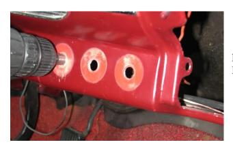
Locate the (3) holes next to the glove box opening. Drill these holes to 7/16" dia.
