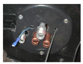
Locate the Firewall Block Off plate, and (3)  $\#10 \times 3/4$ " hex head tek screws.
