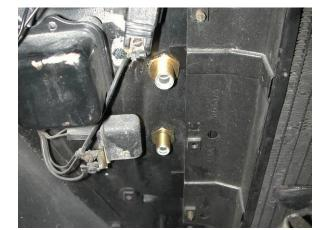
Reinstall tubes to the condenser using a few drops of mineral oil at each of the connections.
