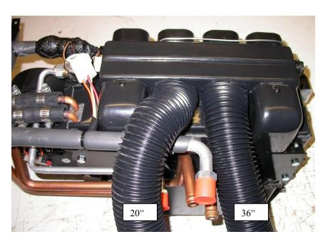
Locate the Evaporator, (1) piece of 2" dia. Flex hose 20" long, and (1) piece of 2" die flex hose 36" long.
