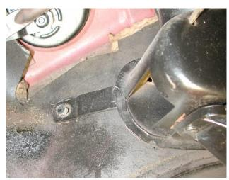
Locate on drivers side of the heater (1) bolt that attaches ducts to the firewall.
