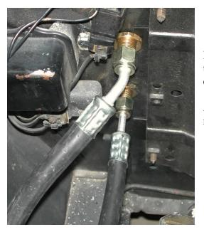
Locate the Discharge Hose from the condenser kit. Attach to #8 fitting on the radiator bulkhead and route over to the compressor.
