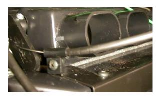
Locate Heat / Defrost cable assembly, and (1)  $\#8 \times 3/8$ " pan head screw. Cable is the one that has wire off set and cable attachment lug.
