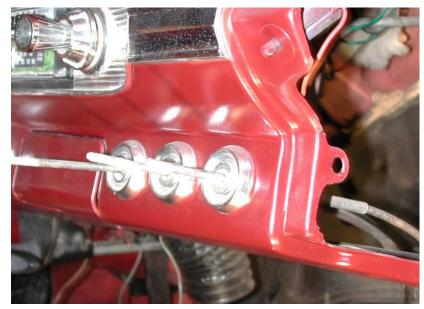
Remove (3) control cables and knobs from instrument panel and discard the cable and switch.
