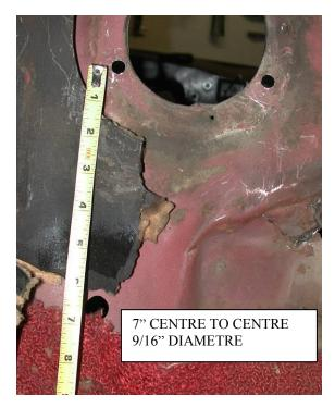
Locate behind glove box and on firewall the hole that previously mounted the heater box. Locate and drill (1) 9/16" dia. hole for the drain tube 7" directly below the original hole as shown.
