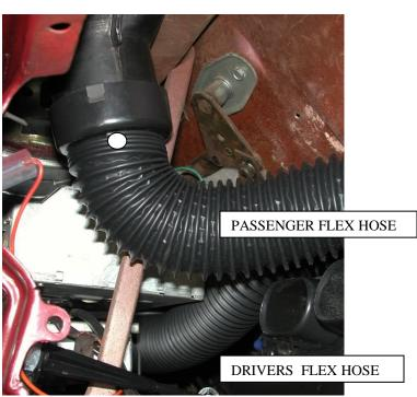
The 20" flex hose that was attached to the defrost outlet on top of the evaporator attaches to the passenger defrost diffuser.
