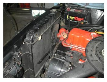
.Remove radiator fan, and the radiator. Retain all of original hardware.
