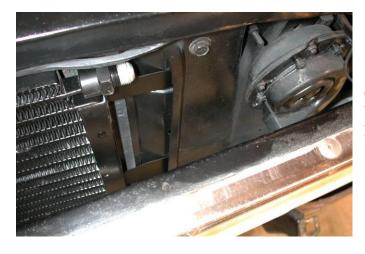
Condenser is inserted from the engine side of the bulkhead. Reinstall radiator using the original hardware.
