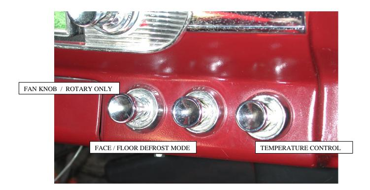
THE PICTURE YOU SEE ON THE FIRST PAGE SHOWS THE CONTROLS IN THE FACE MODE. THIS MEANS THAT THE AIR WILL BE DISTRIBUTED THROUGH THE FACE OUTLETS. THIS ALSO HAS THE TEMPERATURE KNOB IN THE COLD POSITION. WITH THE CONTROLS IN THIS POSITION YOU WILL GET THE AIR THROUGH THE FACE OUTLETS WITH THE COMPRESSOR ON.
