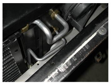
Locate Discharge Tube and the Liquid Tube Assembly.
