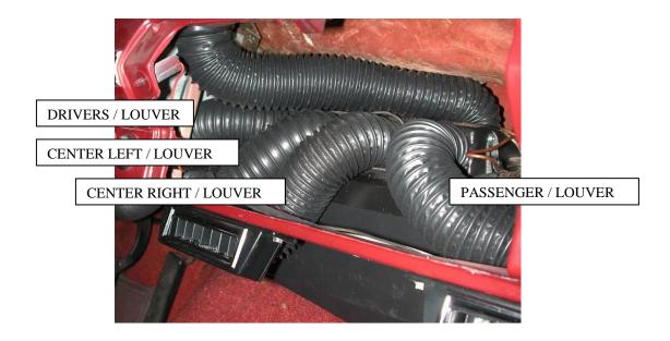
Locate 2" Dia. flex hose Cut (1) piece 36" long. Attach to face duct over the left outlet. Route behind instrument panel over the unit brace and steering column and attach to the drivers louver.
