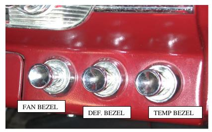
Locate in the Control Sak Kit (1) cable assembly and (1) blower switch assembly.
