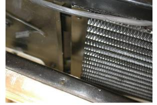
Condenser brackets are clamped between the radiator mounting flange and radiator bulkhead.
