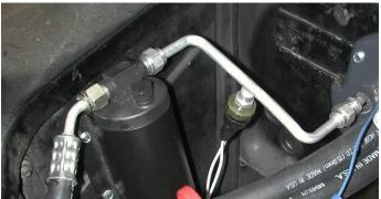
Attach drier assembly to inner fender using liquid tube as a guide. Attach using (2) #10 tek screws.
