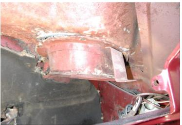
Locate behind glove box opening the air inlet flange.
