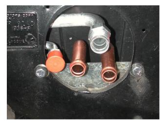
Attach unit to the firewall using (2) 1/4"-20 x 1" hex head screws and # 1/4" SAE washers.
