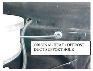
Locate Temperature Cable attached to the control head. Route this cable straight towards firewall and out through original hole that supported the original heater and defrost ducts.
