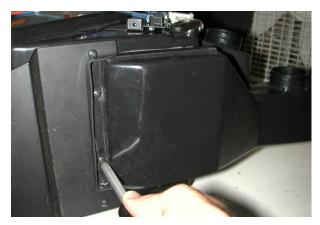
Locate Defrost / Heat duct and (2) #10 x 5/8" pan head screws.
