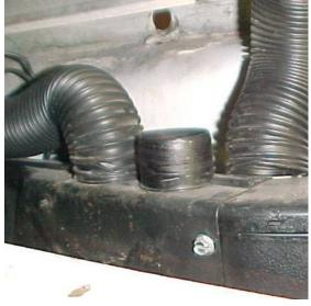
Locate on front of the heater assembly (2) screws that hold heater to the distribution assembly.
