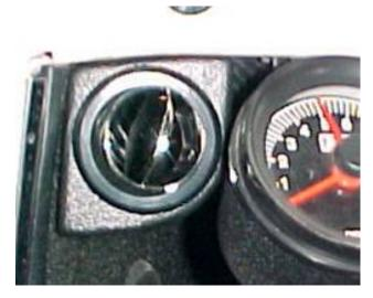
Locate drivers side louver. Remove ball louver and attach housing to the drivers side instrument panel using (2) #10 x 3/4" Tek screws.
