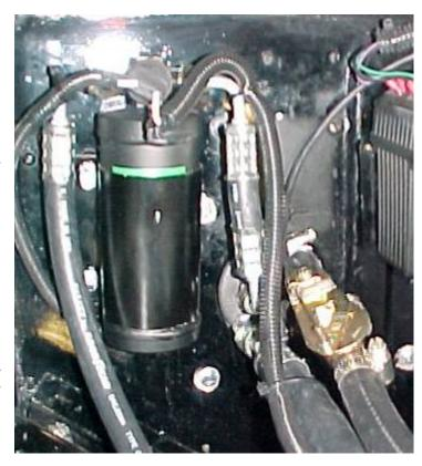
It is recommended that the heater hoses be replaced at this time. Hookup the heater hoses to the connections coming through the firewall. NOTE: SUPPLY LINE FROM ENGINE WILL BE HOOKED TO THE LOWER FITTING USING A WORM GEAR CLAMP.
