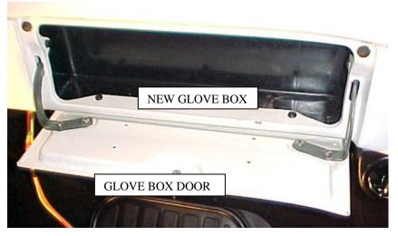
Locate New Glove Box and install into the opening using original hardware.
