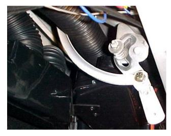
Route flex hose from drivers louver up and behind instruments and then through center of Fresh Air Vent lever then down and connect to center outlet on the Center Duct assembly
