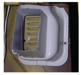
If vehicle is equipped with the deluxe heater. Remove the air inlet box from the passenger side.
