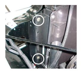
Locate Condenser, (2) Left side, (2) Right side condenser mounting brackets, Liquid Hose (Condenser to Bulkhead), and Discharge Hose (Condenser to Bulkhead). Attach these components on condenser as shown. Use (8) #10 x 3/8" hex head screws. Use (1) #6 o-ring, (1) #8 o-ring and a few drops of mineral oil.
