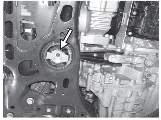
3) Lubricate the APR subframe mount insert with a silicone-based spray or grease. Push the APR insert into the subframe mount as shown, filling in the open gaps in the factory mount.
