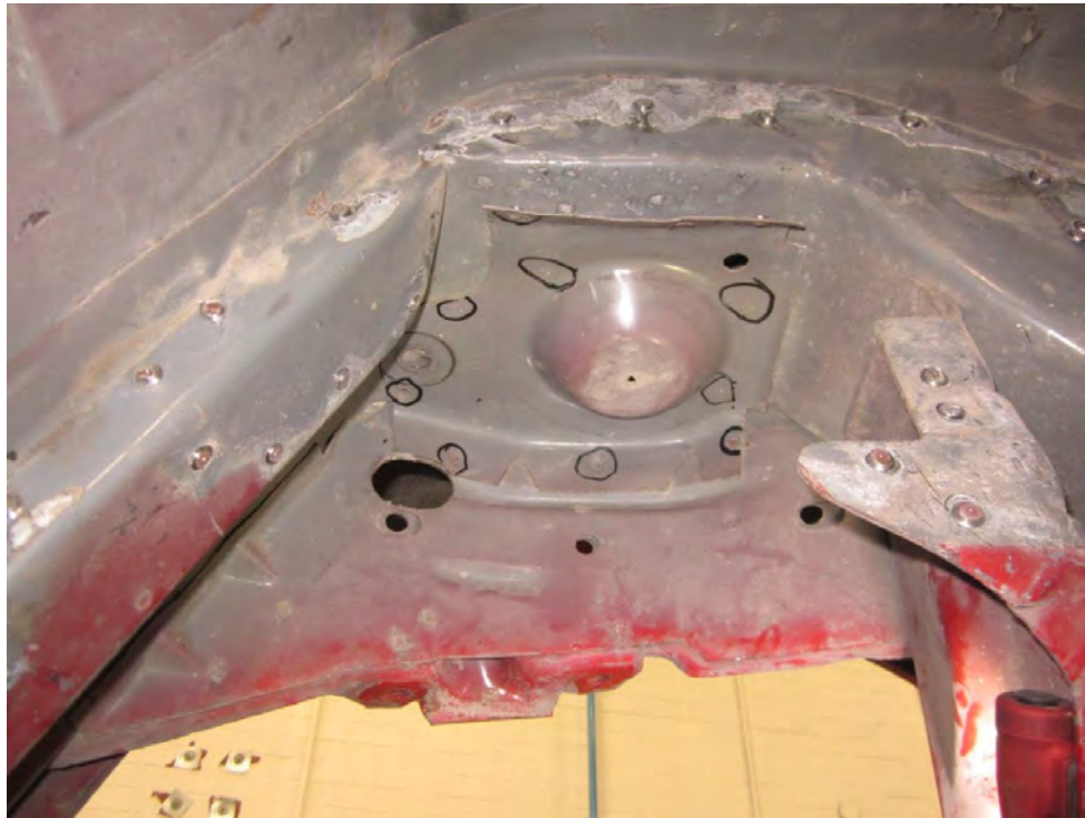
Inner Rail Panel, Removed, Figure 5
