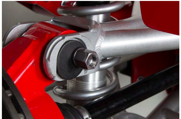
Cam Bolt installed, Figure 59
