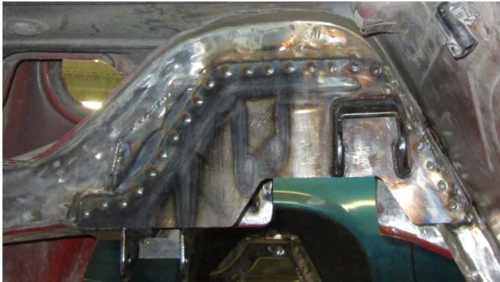
Welded Drivers Side Saddle, Figure 26a
