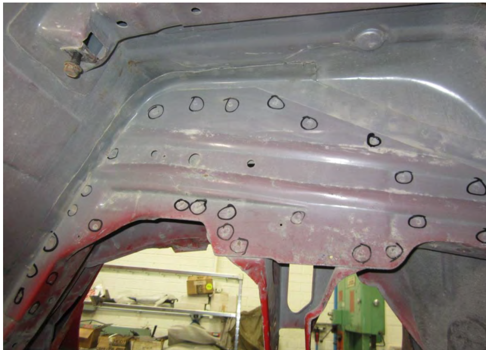
Passenger Side Inner Frame Rails, Mark Spot Welds, Figure 4
