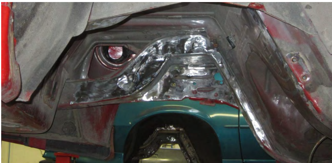
Drivers Side Frame Rail, Spot Weld Holes Filled Figure 12
