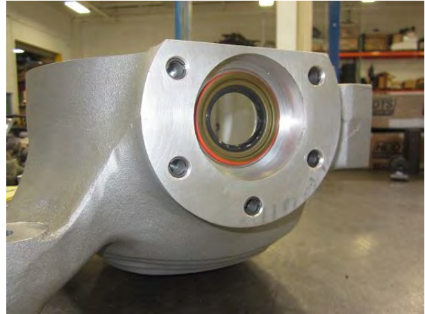
Axle Seal Installed, Figure 28
