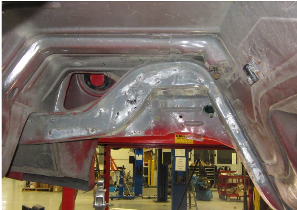
Drivers Side, Inner Panel Ribbing Removed, Figure 11
