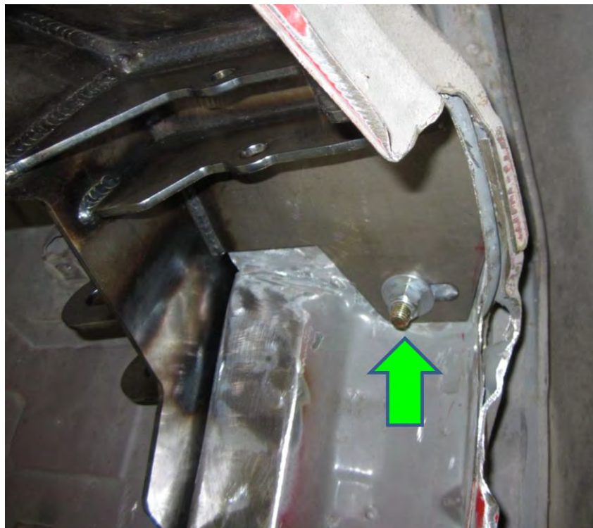
Install 1/2" Bolt to position Saddle in place, Figure 23
