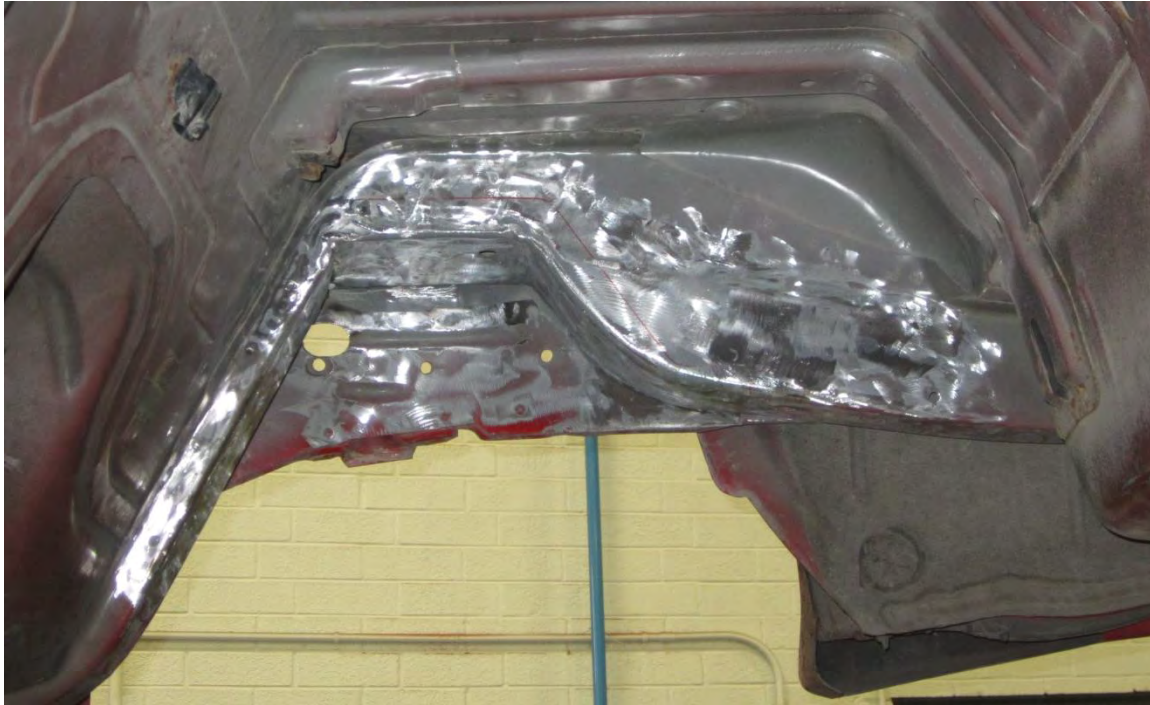
Passenger Side Frame Rail, Spot Hole Welds Filled, Figure 13
