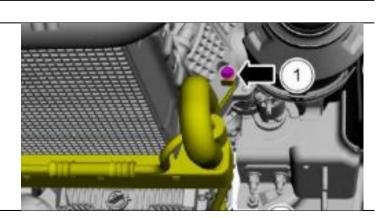
Reconnect driver's side coolant tube retainer.
