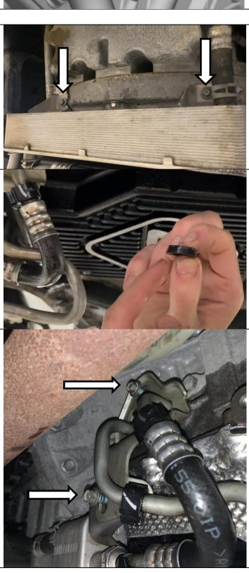
Reinstall the 4 stabilizer bar bracket nuts.
