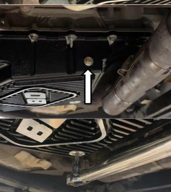
Install the heat shields back on to the studs. Torque the 6 nuts to **80 in-lbs.**
