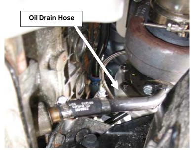
turbo, making sure that it points towards the engine with the compressor housing facing forward.
