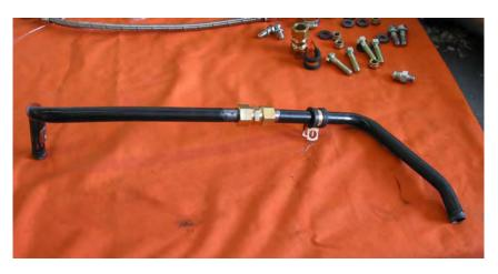
manifold and hook it back up to the factory rubber hoses. Once positioned, tighten the brass coupler and install the new support clamp to the oil filter housing bolt. Zap strap the two rubber heater hoses to secure them together.
