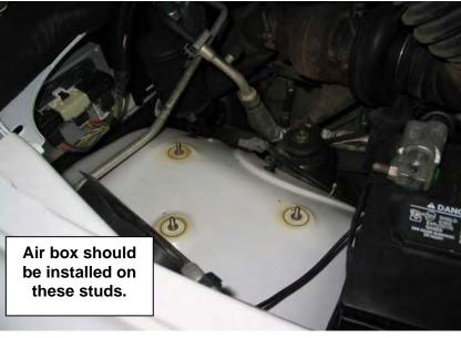
compressor-housing inlet of the *primary turbo*. Install air box onto the factory BD ENGINE BRAKE, INC.
