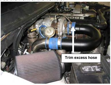
pipe to the *primary turbo* using the supplied V-band clamp.
