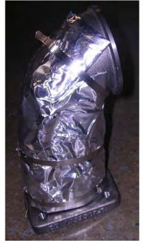
28. You can know bolt the flanged turbine adapter to the primary turbo. Use the four M10x1.25x30 FINE threaded bolts and washers to secure the two. At the same time mount the SS primary turbo support bracket to the assembly.
