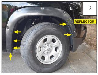
Reinstall (6) factory screws. Apply side reflector (LT1-0002).
