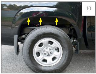
**NOTE:** For short bed installation only: Inspect rear wheel well and note that there are (3) square holes at the top. On Pro4X models there will be (3) screws in this location that need to be removed. Proceed to **Step 12.**
