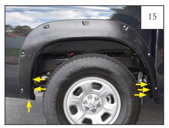
Reinstall (6) factory screws. Rear flare installation complete. Repeat for opposite side.
