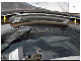
Install bracket using using (2) previously removed screws.
