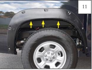
**NOTE:** For long bed installation only: Hold flare in position and mark (3) locations where holes in flare align with truck fenderwell. Mark these locations with a grease pencil. Proceed to **Step 12**.
