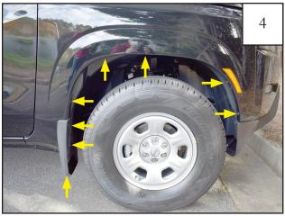
Remove (8) factory installed Phillips screws. Retain screws as these will be reused to install the new flare.
