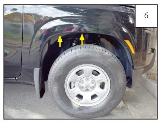
Locate (2) holes at the top of the wheel well.
