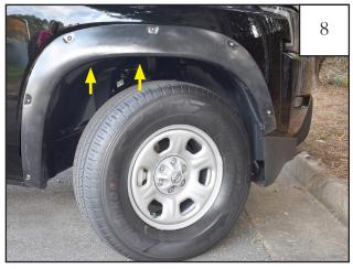
Place fender flare on vehicle and align with holes. Install (2) SW1-0058 Phillips Truss Screws in the locations where the bracket was installed in **Step 7**.
