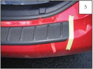
Hold the part at an angle to prevent tape from prematurely sticking, and align the part on the bumper by aligning center rib in part with metal loop on striker and using the masking tape applied in Step 2 as a guide.
