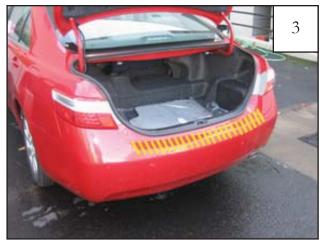
Make sure that all installation surfaces are free of dirt and/or grease. Use a clean, lint-free cloth and isopropyl alcohol-based cleaner.
