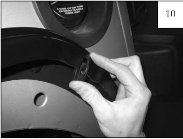
Install supplied "U" Nuts, with the thread side in, over holes in Inner Flare Piece (8 places).
