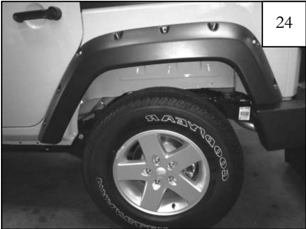
Ensure fit, and tighten all screws
