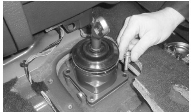
14. Install the B&M shifter using the stock screws. Tighten the screws to 17 ft-lbs torque.
