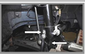
Remove the strut tower brace is applicable. Starting with either driver side or passenger side remove the wheel. Disconnect the brake line bracket and detach the ABS sensor wire from the strut body.
