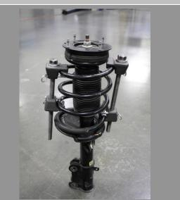
With a spring compressor, slowly depress the spring, then remove the upper strut retaining nut, then remove the upper strut mount assembly from the strut shaft. <u>NOTE!!!</u> Recommend the use of an impact gun.
