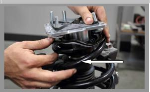
Place the Camber/Caster Assembly onto the Strut Assembly. NOTE III There is a supplied spacer for the 2005-2010 Mustang GT Models that needs to be placed onto the strut shaft before sliding the Camber/Caster Plate on.
