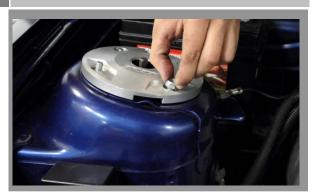
Re-install the strut assembly, place the cover over the strut tower where the studs protrude, don't fully tighten the top nuts. The factory strut tower brace can be used with this kit by placing the 2 ends above the decorative cover. NOTE!!!Remember to remove the rubber band holding the Camber/Caster Kit.
