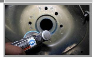
Check the bottom of the strut tower housing for any roughness. Use a Sander or sand paper to smooth out the Housing. NOTE !!! Must be smooth to allow the Camber/Caster Assembly to slide freely when adjusting.
