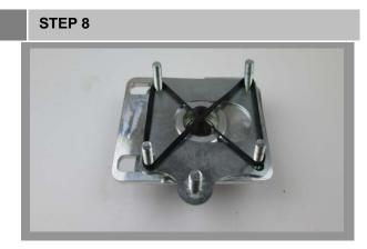
Place the Caster Plate on top of the bearing plate. Make sure that the raised lip around the bearing plate protrudes up through the center slot of the Caster Plate. <u>NOTE!!!</u> The use of a rubber band will help hold the stud plates in position while installing. Be sure the plates move from side to side smoothly.
