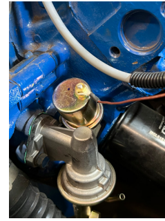
Oil pressure sender installed into the 1/4"NPT extension.
