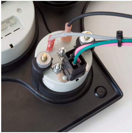
View of wire harnesses installed, connected to gauges.
