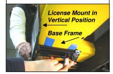
B. When the bottom of the bumper is deep enough, the base can be simply mounted using three screws
