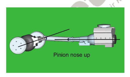
How do you set the pinion angle? On a single-piece shaft you want to set it up where a line drawn through the center of the engine crankshaft or output shaft of the transmission and a line drawn through the center of the pinion are parallel to each other but not the same line.
