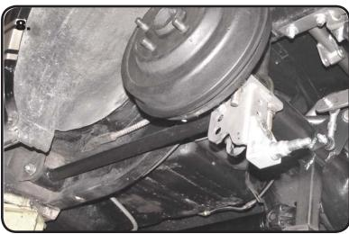
**8.** Install the Lower Bars with the Grease Zerk pointing down. The bar is attached to the Axle Mount in the **TOP HOLE** using (1) 5/8" x 2 3/4" Hex Bolt, and (1) 5/8" Thin Nylok Jam Nut. The front of the Lower Bar is attached with 1/2"x 6" Hex Bolt(64-67) or 1/2"x 4 1/2"Hex Bolt(68-70), and (1) 1/2" Nylok Nut.
