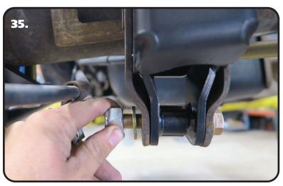
**35.** Install a 9/16" SAE flat washer on a 9/16"-18 x 3 1/2" bolt. Insert the bolt through the OEM lower shock mount and panhard bar bracket. Install a 9/16" flat washer and 9/16"-18 nylok nut on the threads of the bolt. Do not tighten the hardware at this time.
