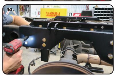
**14.** Tighten all of the c-notch side bolts. Torque to 50 ftlbs.
