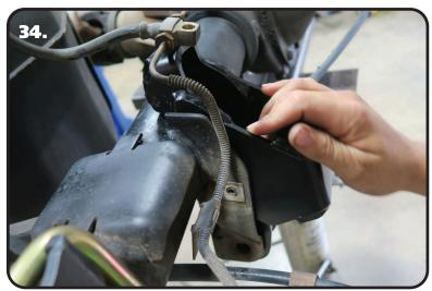
**34.** Position the panhard mount in the driver side shock bracket. The bottom mounting hole of the panhard bracket will align with the factory shock mounting hole.
