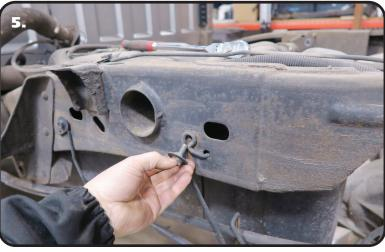
**5.** Unbolt the emergency brake cable bracket from the driver side frame rail. It is located between the axle and the front leaf spring hanger. Retain the hardware for reassembly.
