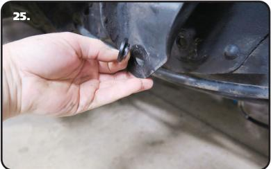
**25.** The kit includes (4) t-busings for the front leaf spring mount. Insert a t-bushing in each front leaf spring mounting hole with the small OD inserted into the hole. The large OD needs to be on the oustide of the brackets.
