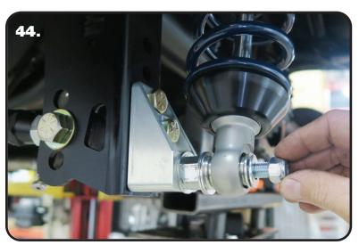
**44.** Install the 7/16" Flat washer and 7/16" Nylok nut. Tighten the upper and lower shock bolts. Torque the Upper Bolt to 50 ftlbs and the Lower Nut to 40 ftlbs. The designed ride height of the CoilOver/Shockwave is 14 1/2" center to center.
