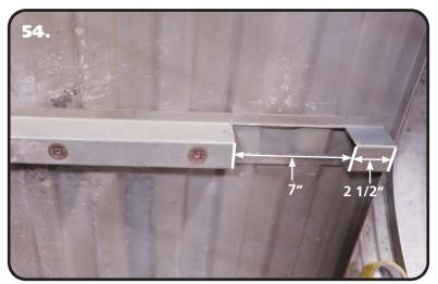
**54.** Trimming of the bed brace that is in between the wheel wells is necessary to clear the c-notches and wishbone. We cut ours with a die-grinder. **Image 54** shows the passenger side, the dimensions are the same for both driver and passenger. The first notch starts 2 1/2" from the end of the brace. The notch is 7" long. Trim the driver and passenger side using these dimensions. **Image 55** shows the driver and passenger sides cut out.
