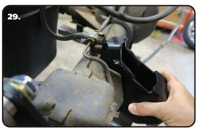
**29.** Depending on the year of your truck, it may have the rear brake hose attached to the axle above the driver side shock mount. If your truck doesn't have the brake line mounted in this location, skip to **Step 33**. If your truck has the brake line mounted in this location, continue to **Step 30**.
