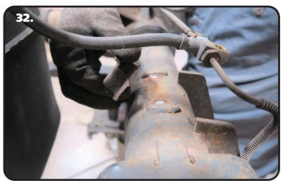
**32.** With both sides of the bracket cut, remove it from the axle tube. Grind the area smooth.
