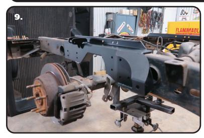
**9.** After cutting, slip the c-notch over the frame to check the fitment.
