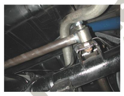
10. Replace the factory panhard bar with the new one using the new stud and hardware supplied. The rubber rod end will be attached to the axle.
