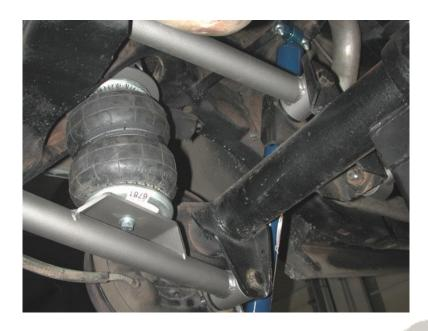
1. Replace the factory upper trailing arm with the StrongArms. 5/8" x 3 3/4" bolts and Nylok jam nuts are supplied to replace the factory hardware. An aluminum spacer will be installed on each side of the Heim end.
