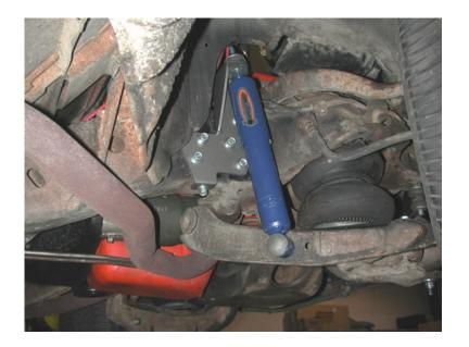
6. To correct the sway bar alignment the endlink must be shorten to 2" tall. A 3/8" x 6  $\frac{1}{2}$ " bolt is supplied.
