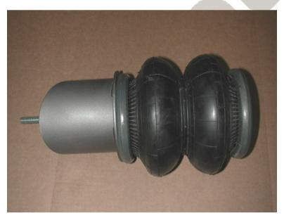
3. Bolt the lower air spring plate to the lower arm. The two outer holes will align with the factory bump stop holes. The inner two holes must be drilled.
