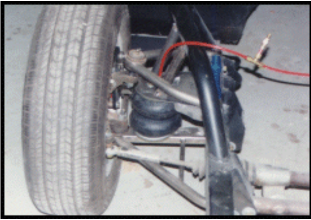
Aftermarket Mustang II installation [replaces coilover shock]
