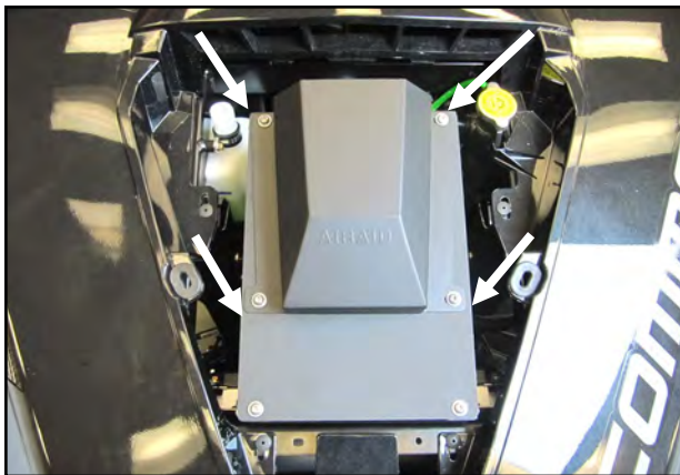
20. Mount the Hood Scoop onto the Airbox assembly a shown using four sets of 1/4-20 Button Heads and Washers. Leave the Screws Finger Tight for now.
