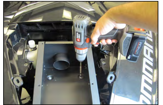
15. Using the drill and a 8mm socket, drive the Self Drilling Screws (#15) with a 1/4" Flat Washer into the cross member.
