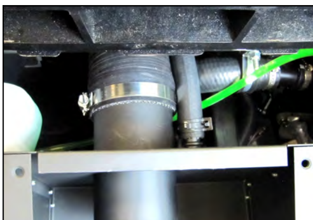
17. Close up view of rerouted PCV hose. Note that the factory spring clamp is reused.
