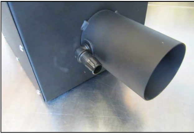
10. Install the Grommet (#10) and Elbow Fitting (#11) into the Airbox Tube.
