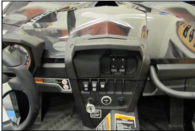
29. Reinstall the center console using the factory hardware and reconnect the battery.
