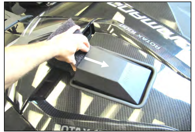
27. Compress and install the Foam Pre Filter (#7) into the Hood Scoop.
