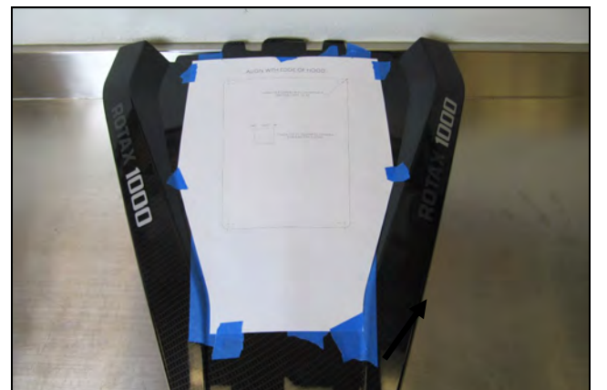
21. Prepare the hood for cutting by laying tape strips side by side all across the center section for scratch protection. Cut out the template and tape it into position.
