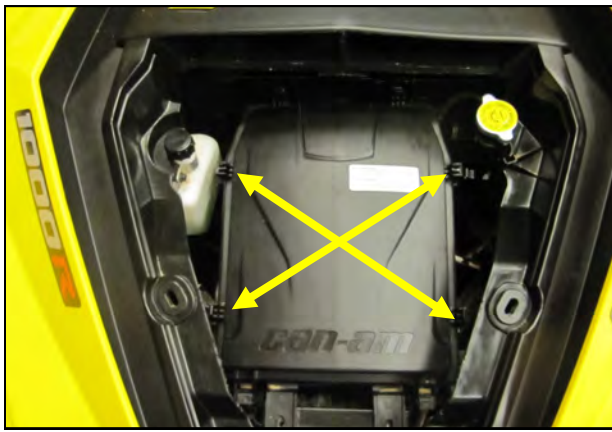
11. Unclip the upper half of the airbox and remove it along with the air filter.
