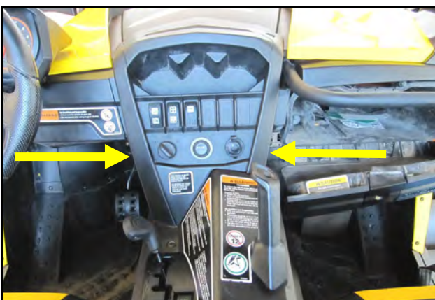
4. Open the glove box and remove the two plastic rivets on each side the center console.
