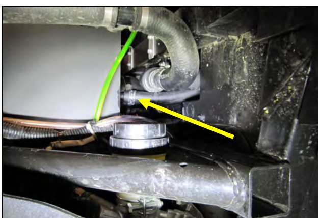
32. Connect the PCV line to the Elbow Fitting on the Intake. Note that the factory spring clamp is reused.
