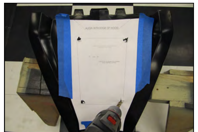
36. Prepare the hood for cutting by laying tape strips side by side all across the center section for scratch protection. Cut out the Template and tape it into position. Using a 1/8" bit, drill out four pilot holes in the hood followed by a 1/2" bit to finish.
