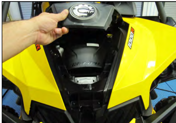
2. Remove the center section of the hood to gain access to the airbox assembly.
