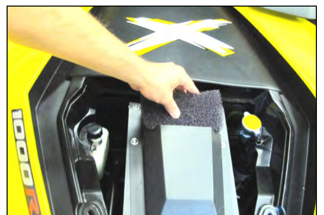
39. Compress and install the Foam Pre Filter (#7) into the Hood Scoop.
