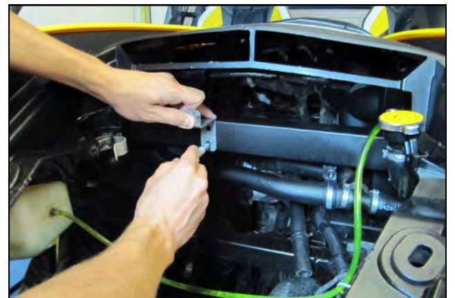
18. Using one of the Rear Brackets (#11) and a spring loaded punch, mark the cross member at both 3\"/>
