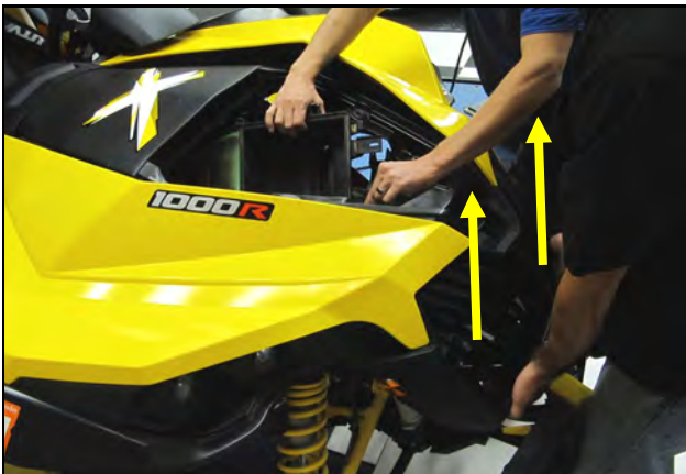
16. With the help of an assistant, lift the front plastic away from the vehicle and remove the lower half of the airbox.
