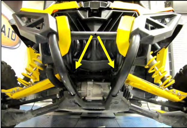
13. Remove the two 8mm nuts and bolts in the upper bumper mounts.
