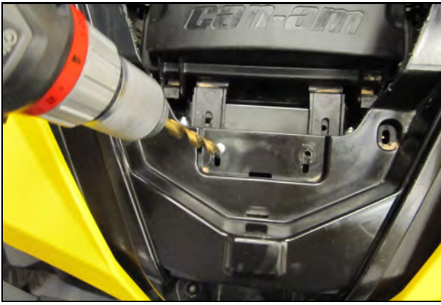
10. Drill out the rivet heads holding plastic to the core support.
