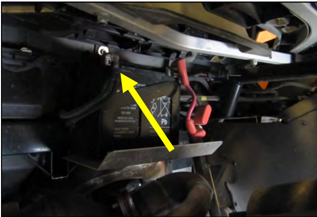
1. Disconnect The Negative Battery Terminal. It is located above the exhaust, in the rear of the vehicle.
