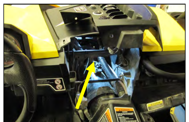
6. Loosen throttlebody clamp .
