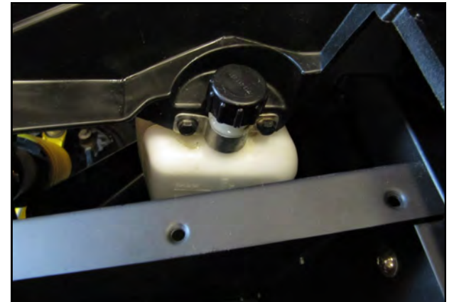
30. Reinstall the coolant bottle.
