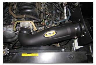
**10.** Install the Airaid Intake Tube into the Hump Hose first, and then press the reducer onto the throttle body. Adjust for fit, and tighten all four Hose Clamps.
