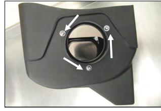
4. Install the Filter Adapter (#4) onto the Cold Air Box
