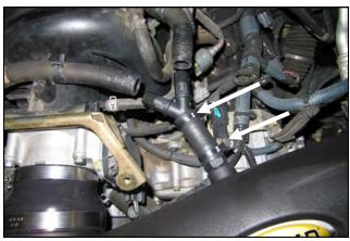
**11.** Install the 5/8" Hose (#16) onto the Barbed fitting in the Intake Tube. Insert the Barbed "Y" Fitting (#14) into the 5/8" Hose and secure using the two Speed Clamps (#17).
