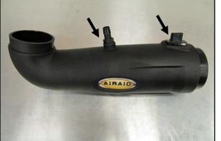
7. Install the threaded 5/8" Barbed Fitting (#15) into the Airaid Intake Tube (#2). Transfer the Mass Air Flow sensor from the factory airbox, into the Airaid Intake Tube and secure using the two 8-32 Button Head Screws. Do not attempt to reuse the factory screws. Apply the Airaid Decal to the Tube as shown.
