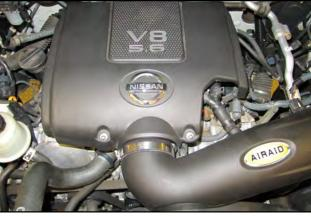
17. Reinstall the engine cover in the reverse order in which it was removed, rear first, front last. Only now it is to be secured using the two Acorn Nuts (#11) and two 1/4" flat washers.
