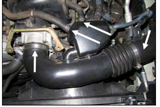
2. A.) Using a pair of pliers, compress the spring clamps on the PCV breathers and then slide back. Disconnect the breathers from the factory intakeB.) Loosen the two clamps on the factory intake tube and remove it from the vehicle.
