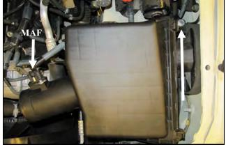
**3.** Disconnect the Mass Air Flow sensor, or MAF, and separate the wiring harness from the airbox lid. Using a 10mm socket, remove the single bolt securing the airbox. Lift straight up on the airbox assembly and unseat it from the mounting grommets on the inner fender. 4WD models will need the differential breather disconnected from the airbox lid.
