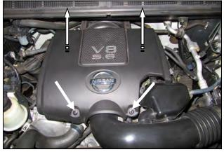
**Disconnect The Negative Battery Terminal! 1.** Using a 10mm socket, remove the two front engine cover bolts. Lift straight up on the cover and unseat the rear half from it's mounting grommets.
