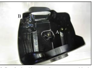
5. Transfer the airbox mounting grommets and hard-
