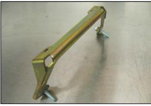
**14.** Remove the factory engine cover mounting bracket from the intake manifold and install the two 6mm x30mm Bolts (#10) as shown. They are to be installed from behind and protrude forward when installed properly.
