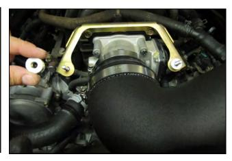
**15.** Reinstall the bracket onto the intake manifold and place a Spacer (#13) onto each 6mm bolt.
