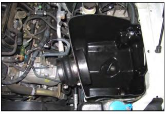
**9.** Slide the Hump Hose (#6) and #72 Hose Clamps (#20) onto the Filter Adapter. Leave the clamps loose for now.
