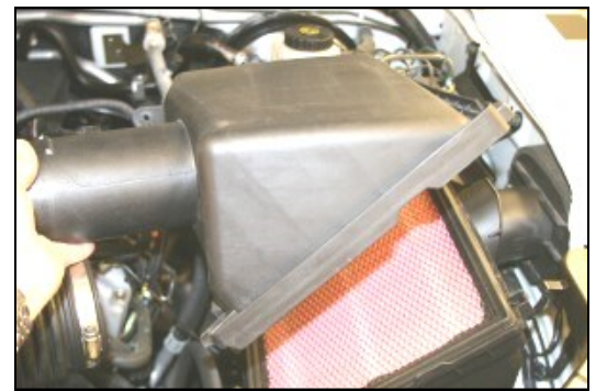
6. Remove the factory airbox lid.
