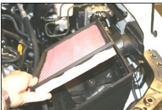
7. Remove the factory air filter.
