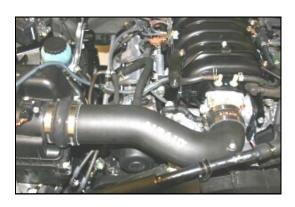
9. Install the MIT into the hump hose first, and then into the reducing coupler. Adjust the MIT snugly against the throttle body, and tighten the 4 hose clamps. Next install the 1/4 - 20 x 1/2" button head bolt (#10) and 1/4" flat washer (#11) thru the Adel clamp and into the MIT to hold the air conditioning hose.
