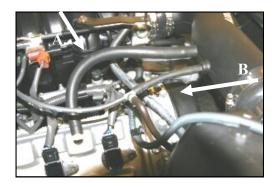
**10.** A) Install the 1/2"x 13" breather hose (#5) from the **MIT** to the valve cover. B) Install the 1/4" x 1/4" x 1/8" vacuum tee (#12) into the 1/4" x 4" hose (#9) and then to the factory 1/4" and 1/8" vacuum lines, as shown.
