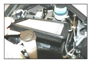
**6.** Remove the factory air filter, and install the Airaid Premium Filter (#1). Reinstall the factory airbox lid, and relatch the 4 clips.
