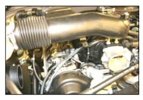
**4.** Remove the factory intake tube from the vehicle
