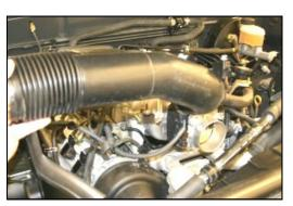
12. Remove the factory intake tube.
