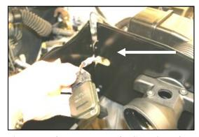
**6.** Remove the top screw on the **CAD**. Spread the panels slightly, and slip the wiring harness thru the gap into the access hole, as shown. Reinstall the screw and tighten.
