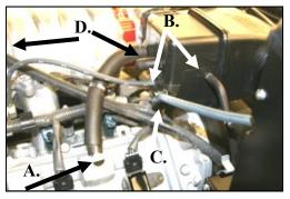
11. A) Disconnect breather hose at the valve cover. B) Disconnect 1/4" and 1/8" vacuum lines on the back of the factory intake tube. C) Unclip MAF wire harness retainer from the intake tube. D) 01-03 Sequoias and 00-02 Tundras only; remove 3/8" vacuum hose between factory intake tube and metal fitting on top of the intake manifold. (Hose Not Shown)
