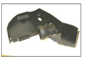
**3.** Assemble the Airaid Cool Air Dam (CAD) panels (#2, #3) using three 6-32 x 5/16" screws (#17), #6 flat washers (#18), and 6-32 keps nuts (#19). Install the MAF adapter (#4) using two 1/4 - 20 button head bolts (#20), and 1/4" flat washers (#21), as shown.
