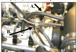
**16. 03-04 Tundra, 04 Sequoia**A) Install the 1/2"x13" breather hose (#8) from the **MIT** to the valve cover. B) Install the 1/4" x 1/4" x 1/8" vacuum tee (#15) into the 1/4" x 4" hose (#16) and then into the factory 1/4" vacuum hose, and 1/8" vacuum hose as shown. Refer to the hoses in step #11. Reinstall the beauty cover from step #10
