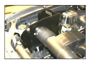
**5.** Slide the **MAF** adapter into the factory tube, and at the same time slip the **CAD** onto the top of the factory airbox base, adjust for fit and relatch the 3 factory clips. Tighten the hose clamp on the factory intake tube. Reinstall the shroud bolt from step #4.
