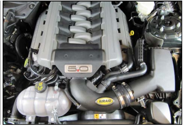
12. Double check your work. Make sure all clamps, hoses, bolts, and screws are tight. Double check the hood clearance. Reconnect the negative battery cable and reinstall the cover.
