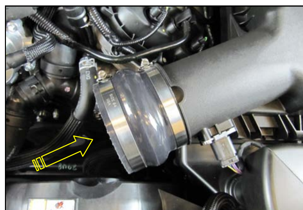
5. Slide the Hump Hose and Clamps onto the airbox outlet as shown. Do not tighten the clamps at this time.
