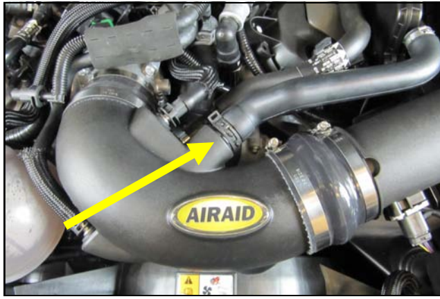
11. Connect the resonator to the Intake Tube as shown
