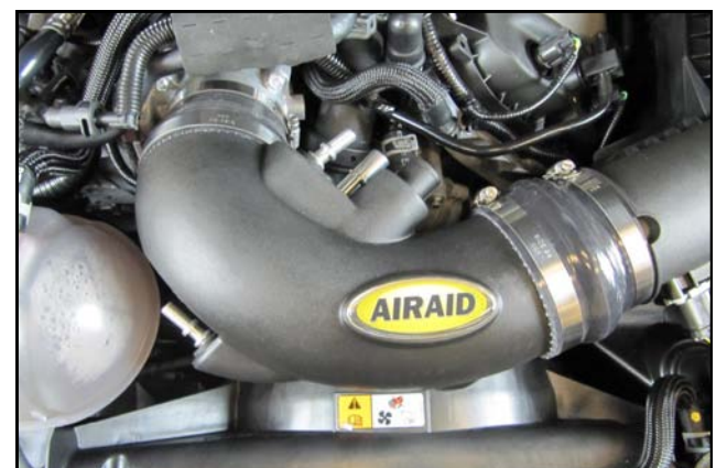
9. Insert the Intake Tube into the Hump Hose and Reducer then tighten all 4 Intake Clamps.
