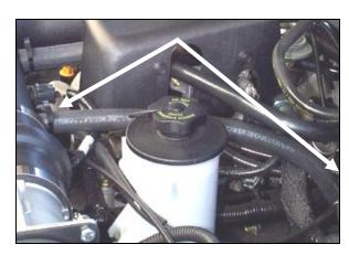
**12.** Install the 5/8"X18" breather hose (#6) onto the valve cover breather fitting then onto the Airaid Intake Tube nipple. Secure the hose using two #19 speed clamps (#16).
