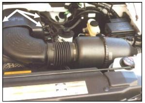
1. <u>Disconnect the negative battery cable.</u>
