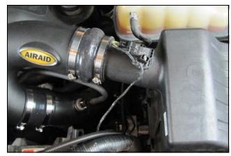
**9.** Reconnect the air meter or Map sensor and tighten all Clamps.
