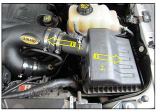
**8.** Slide the Hump Hose onto the Airaid Intake tube as far as it will go then insert the air box lid tabs into the slots. Adjust the assembly until the lower air box clips can positively engage the lid and lock.
