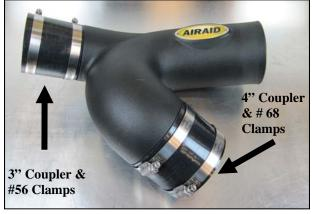
**5.** Slide the Couplers and Clamps onto the Intake tube
