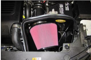
14. Plug the Harness Extension into the factory wire har- 15. Install the Airaid Premium filter onto the Filter onto the top of the Air box as shown, with the contour rolling away from the filter.
