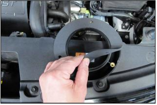
**6.** Prepare the Filter Adapter for installation by position ing the Adapter Gasket on the mounting side and lining
