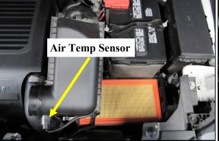
2. Unfasten the factory air box clips and separate the upper half of the air box from the intake assembly. Disconnect the air temperature sensor.
