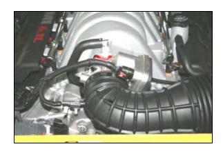
4. Reinstall the factory intake tube, and tighten the hose clamp. Reconnect the Air temperature sensor and throttle body motor. **Re-connect the negative battery cable!**
