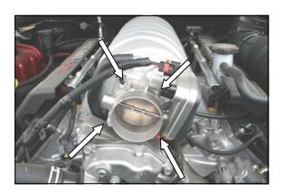
2. Using a 10mm Socket, remove the 4 bolts that hold the throttle body to the intake manifold.
