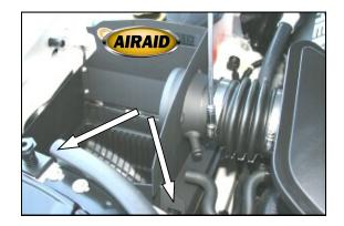
**6.** Install the Quick Fit Panels by sliding the four tabs on the back of the panels into the
