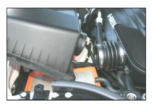
**3.** Remove the factory airbox lid by sliding it forward, and then up and out of the factory intake tube.
