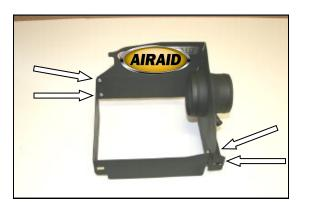
**5.** Assemble the Quick Fit Panels (#2, #3) using four 6-32 x 5/16" screws (#5), #6 flat
