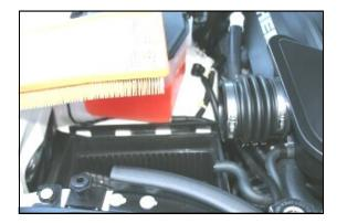
**4.** Remove the factory air filter from the airbox base.
