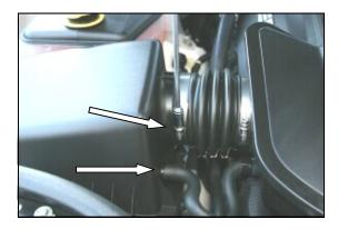
**1.** <u>Disconnect the negative battery cable.</u> Using a 5/16" socket, loosen the hose clamp on the factory airbox lid. Twist and remove the breather hose from the factory airbox lid.
