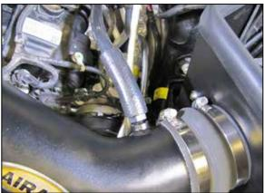
21. Install the provided crank case vent hose onto the fitting installed into the AIRAID® intake tube and then connect the other end to the factory crank case vent tube.
