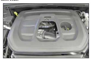
2. Lift up the inspection cover and remove the bolt that secures the decorative engine cover. Then remove the decorative engine cover from the vehicle.
