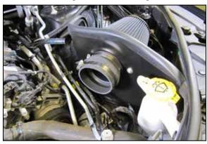
14. Install the heat shield/Air filter assembly onto the air filter housing mounting studs as shown.
