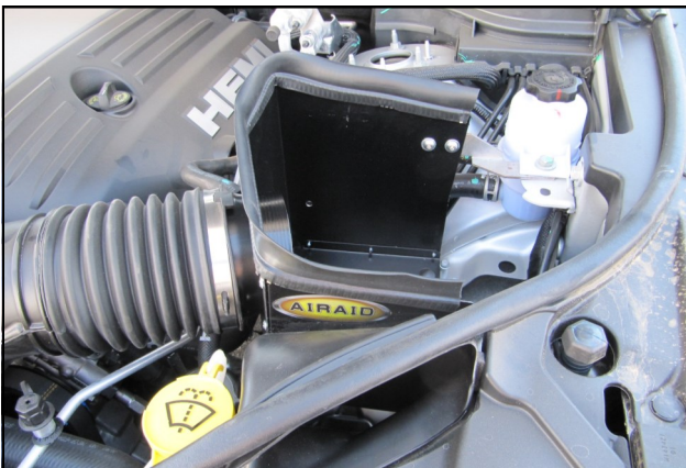
16. Install the Weather Strip (#4) to the top edge of the panels, and reattach the hood seal. Apply the Airaid Decal to the Panel Assembly.
