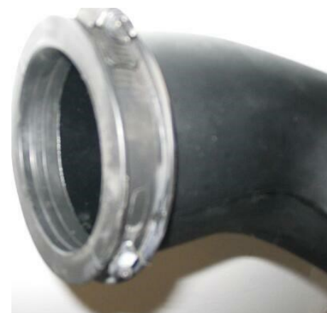
11. Reinstall factory throttle body coupler onto smaller end of intake tube.
