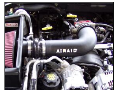
12. Slide the intake tube into the throttle body & align hump hose with Airaid Cool Air Dam. Slide the hump hose over end of the Airaid Cool Air Dam intake and secure using a #56 hose clamp.
