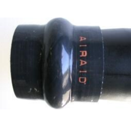
10. Install the urethane hump hose onto larger end of the Airaid Intake tube using the # 56 hose clamp provided.
