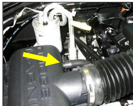
2. Disconnect the crankcase breather tube at the air box lid.
