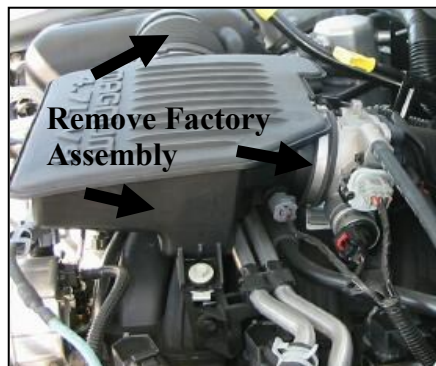
6. Loosen the hose clamp on the throttle body & remove the silencer box & accordion style tube from vehicle.
