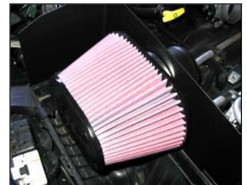
8. Mount the Airaid Premium filter inside the Cool Air Dam and secure with hose clamp provided.
