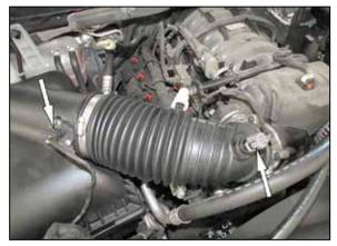
3. Disconnect the inlet air temperature sensor and humidity sensor electrical connections.
