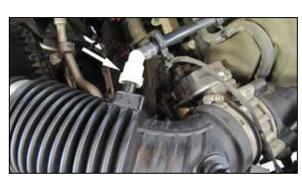
4. Depress the locking tab and then disconnect the crank case vent hose from the factory intake tube.
