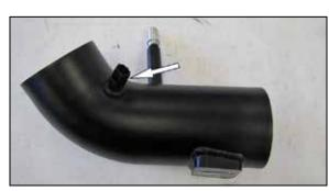
13. Remove the O-ring from the inlet air temperature sensor and then install the sensor into the grommet installed into the intake tube during the previous step.
