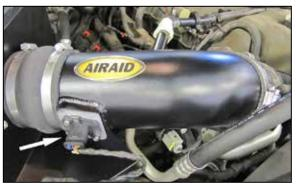
19. Reconnect the humidity sensor and inlet air temperature sensor electrical connections.
