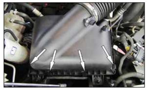
6. Release the four locking tabs securing the air filter housing lid and then remove the housing lid and factory intake tube from the vehicle. Remove the factory air filter.
