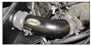
17. Install the intake tube into the hump coupler and then into the step coupler, then adjust the tube for best fit and secure with the provided hose clamps.
