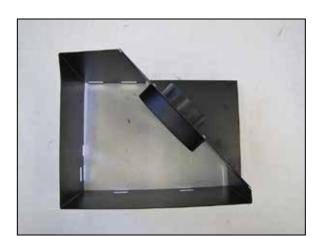
7. Install the filter adapter into the heat shield as shown and secure with the provided hardware.
