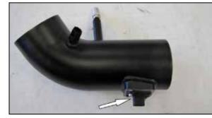
14. Install the humidity sensor into the intake tube and secure with the provided hardware.
