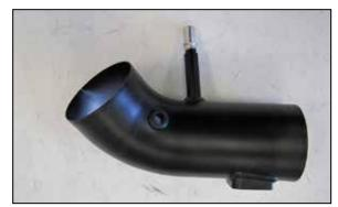
12. Install the provided grommet into the intake tube as shown.
