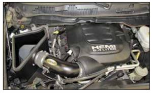
**21. Double check your work!** Make sure there is no foreign material in the intake path. Make sure all clamps, hoses, bolts, and screws are tight. Double check the hood clearance! **Reconnect the negative battery cable!**
