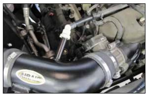
18. Connect the factory crankcase vent hose to the quick disconnect fitting on the AIRAID<sup>®</sup> intake tube.
