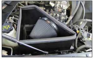
10. Install the heat shield/filter assembly onto the lower air filter housing and secure with the four factory lid retaining clips.
