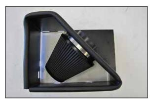
9. Install the AIRAID<sup>®</sup> air filter onto the filter adapter and secure with the provided hose clamp.
