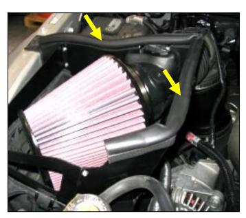
**8.** Mount Airaid Premium Filter to the filter adapter and tighten hose clamp, in addition; press the weather strip onto the top of the Airaid cool air dam. (<u>Hint</u>: start the install at the top corner of the cold air dam & work toward the edges)
