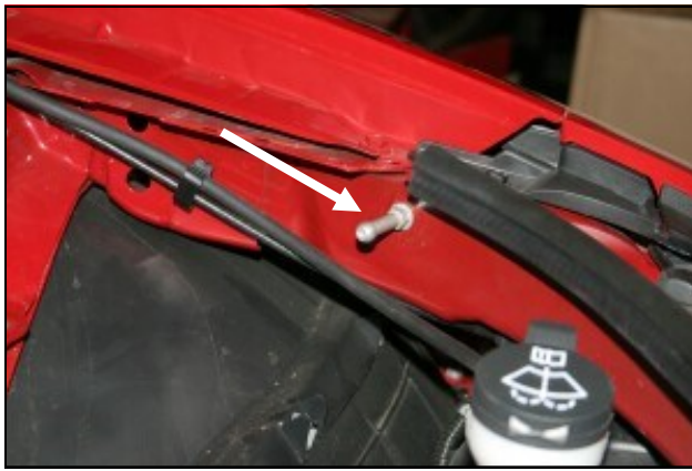
11. Using a 10mm wrench, remove and save the ground lug from the driver's side inner fender. It will be reused in step #13.
