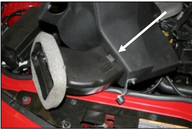
10. Reinstall the factory scoop into the Airaid CAB as shown. It will snap into place.
