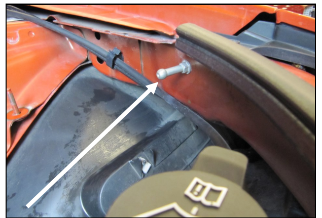
12. Remove and save the ground lug from the driver's side inner fender. It will be reused in step #14.
