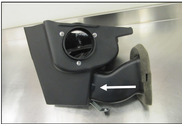
11. Reinstall the factory air scoop into the Airaid Cold Air Box.
