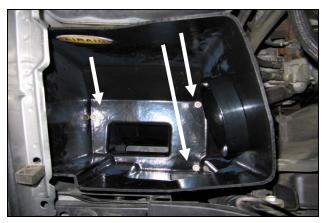
9. Install the CAB into the engine compartment and secure using three of the tray bolts from step 6.
