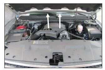
**Disconnect the negative battery cable.** Remove the engine cover by simply pulling up on it and sliding out from the vehicle.
