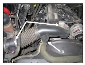
**3.A.)** Loosen the clamps securing the factory intake tube to the throttlebody and the Mass Air Flow Meter,
