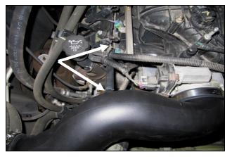
**13.** Install the 3/8" Breather Hose (#7) onto the Barbed fitting and factory hard line.
