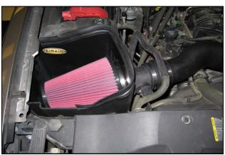
**14.** Install the Airaid Premium Filter (#1) onto the Filter Adapter, and tighten the hose clamp. Install the weather strip (#8) onto the Airaid Cold Air Box. (*Hint*: Start from one corner and work your way around for ease of install.)
