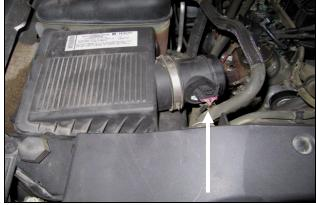
5. Disconnect the MAF sensor and remove the factory airbox and sensor from the vehicle.
