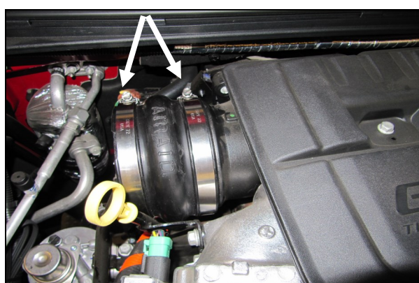
5. Install two #72 hose clamps (#9) onto the urethane hump hose (#4), and then slip the hump hose onto the end of the factory turbo intake tube as shown. Leave the clamps loose for now.
