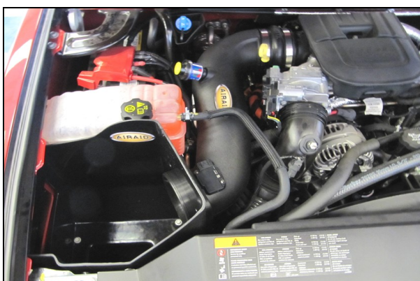
7.) Insert the Airaid Intake Tube into the CAB first, and then into the hump hose.
