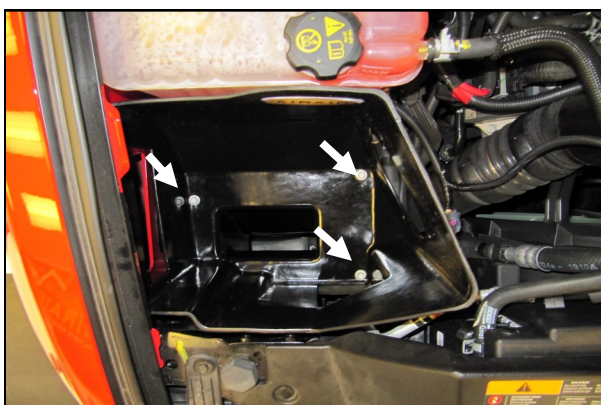
4. Install the Airaid Cool Air Box (CAB) (#3) into the vehicle as shown. Reuse three of the factory bolts from step #3 to fasten the CAB to the inner fender. Leave the bolts loose for now.
