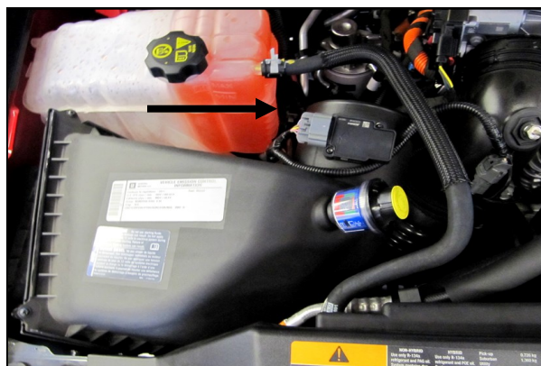
2. Disconnect the Mass Air Flow sensor. Rotate the airbox assembly away from the fender to unseat it from the mounting grommets and remove the entire airbox assembly from the vehicle.
