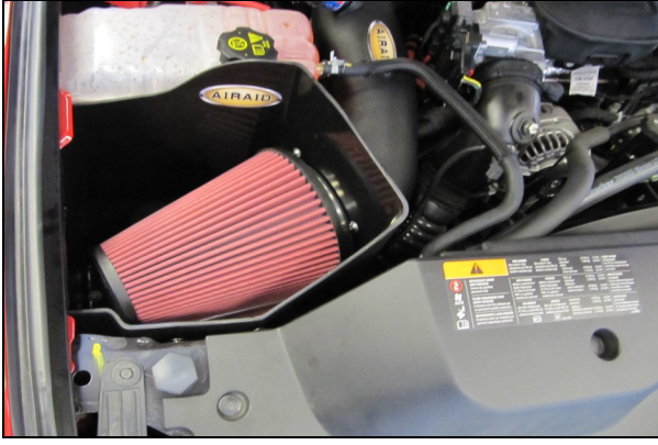
10. Install the Airaid Premium Filter (#1) onto the Intake Tube inside of the CAB.
