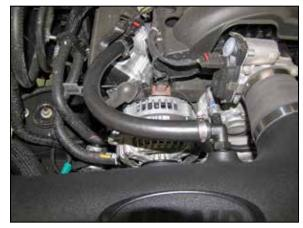
12. Connect the Crank case vent hose quick connect fitting onto the valve cover port and then connect the open end to the fitting installed into the intake tube and secure the hose clamps.
