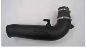
8. Install the provided step coupler (084104) onto the AIRAID<sup>®</sup> intake tube as shown.
