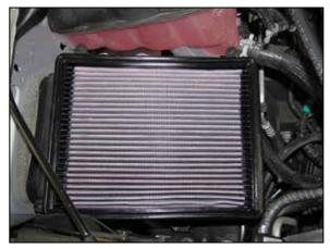
6. Replace the factory air filter with the provided AIRAID<sup>®</sup> air filter and reinstall and secure the upper air filter housing.
