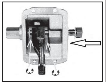
Step 5. Center the slip collar in the axle housing locking both axle halves together. Install the new cover and gasket onto the axle aligning the fork into the slip collar. Sealant is not required on the gasket. Torque the bolts to 10 ft-lbs.
