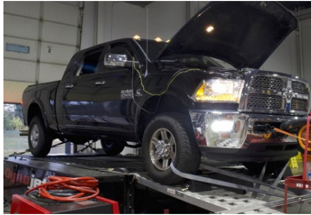
FIGURE 4: A DynoJet™ dynamometer was used for vehicle testing.
