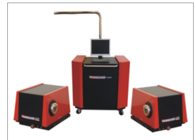
FIGURE 3: A Dynapack dynamometer was used to apply a repeatable load on the Focus ST during testing.
