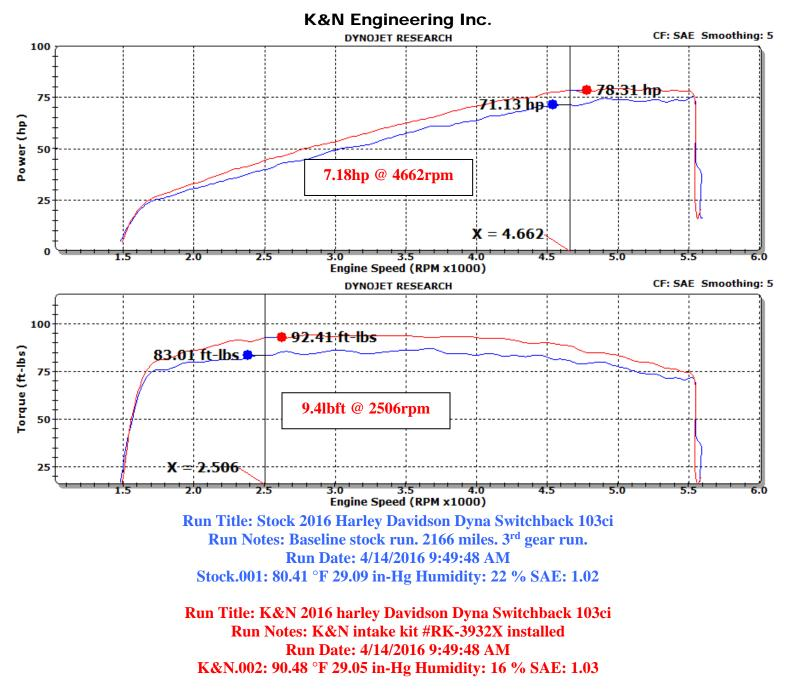
Horsepower gains based on specific or similar vehicle dynamometer test. Results will vary. For more information, lookup vehicle and/or testing protocols at KNFilters.com
