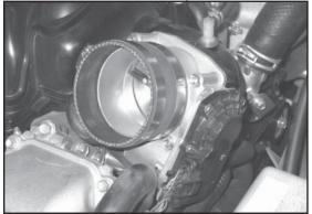
27. Install silicone hose (#08630) onto the throttle body and secure with the provided hose clamp as shown.
