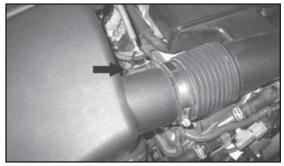
3. Disconnect the mass air sensor electrical connection. Un-hook the wiring harness from the air box. 4. Disconnect the crank case vent hose from the factory intake tube as shown.
