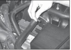
5. Disconnect the fuel pressure regulator vent hose from the factory intake tube as shown.
