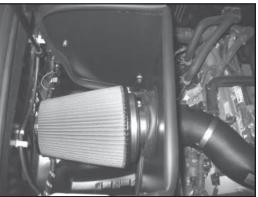
34. Install the K&N air filter assembly onto the K&N intake tube and secure with the provided hose clamp.
