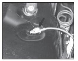
18. Remove the bolt that secures the ground strap to the inner fender.
