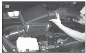
8. Remove the complete factory intake system from the vehicle. Note: K&N recommends that customers do not discard factory air intake.
