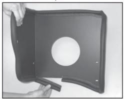
12. Install the large edge trim onto the heat
