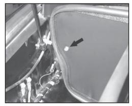
21. Secure the rear heat shield bracket (installed in step #17) to the heat shield with the provided spacer and hardware. **Note: The spacer is to be placed between the heat shield and bracket.**
