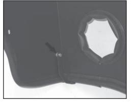
15. Install the small "L" bracket (#07190) onto the heat shield with the provided hardware and spacers as shown. **Note: The spacer is to be installed between the bracket and heat shield.**
