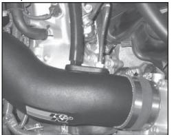
31. Connect the hose mender from the K&N crank case vent hose assembly into the factory crank case vent hose and secure with the factory spring clamp. Then, connect the open end to the K&N intake tube as shown.
