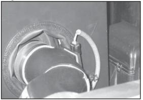
36. Re-connect the mass air sensor electrical connection as shown.
