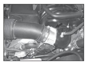
2. Lift the front of the engine cover up, then un-hook it from the rear. Remove it from the vehicle.
