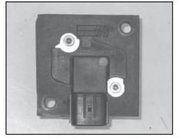
24. Install the mass air sensor into the K&N mass air sensor adaptor and secure with the provided hardware.
