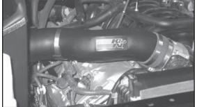
28. Install the K&N intake tube into the silicone hose at the throttle body and align with the saddle bracket installed in step #11. Secure the intake tube with the provided hose clamp.
