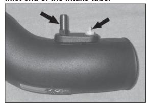
26. Install the provided NPT fittings into the K&N intake tube in the positions shown.
