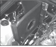
19. Set the heat shield into position on the inner fender. Then, secure the front mounting bracket to the front air box mounting location with the provided hardware.
