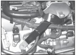
11. Install the tube mounting bracket assembly onto the valve cover using the bolt removed in step #10.
