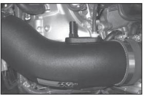
29. Connect the factory fuel pressure vent hose to the K&N intake tube as shown.
