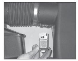
23. Remove the two bolts that secure the mass air sensor into the stock air filter housing. Remove the mass air sensor as shown.
