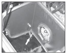
20. Secure the rear lower mounting bracket to the ground strap location with the provided hardware.
