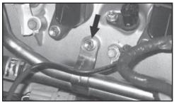
10. Remove the bolt (shown) that secures the engine coolant tube to the valve cover. Note: This bolt will be re-used in the next step.
