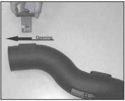
25. Install the mass air sensor assembly into the K&N intake tube and secure with the provided hardware as shown. **Note: The opening in the mass air sensor is to be installed facing towards the inlet end of the intake tube.**
