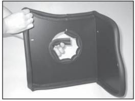
13. Install the small edge trim into the hole of the heat shield as shown.Note: Some trimming of the edge trim may be necessary.
