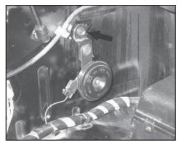
16. On vehicles equipped with a security system horn, remove the bolt that secures the horn to the inner fender.
