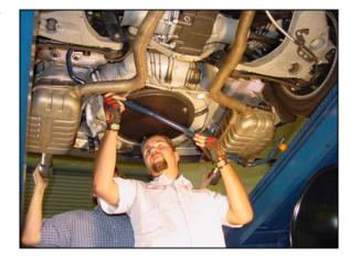
8/ Apply supplied grease to inner-channeled portion of both rear bushings. (approx. half of one tube for rear bushings) Then install the bushings to the bar at approx. the stock location. Position the bar in the stock location then install the brackets over the bushings with the grease fittings pointing down.
