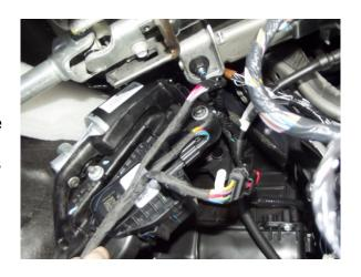
**Step 4:** Secure the PedalMAX unit using the (2) supplied cable ties. The device should not be hanging loosely or unsecured, and should not be mounted to any moving assemblies such as the steering column.
